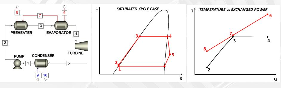
$\Delta T_{\rm PP} {=} T_7 {-} T_3 \text{ PINCH POINT TEMPERATURE DIFFERENCE}$
