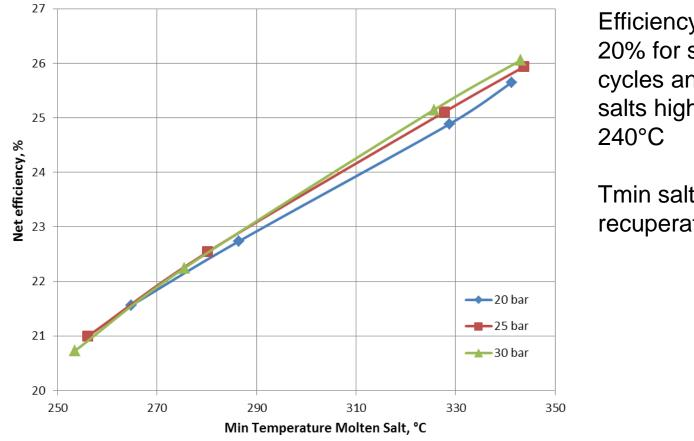
Efficiency higher than 20% for supercritical cycles and Tmin molten salts higher then about
