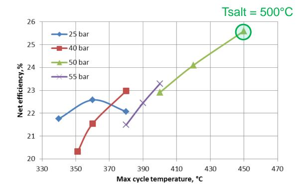
Higher cycle temperatures require higher temperature of molten salts
