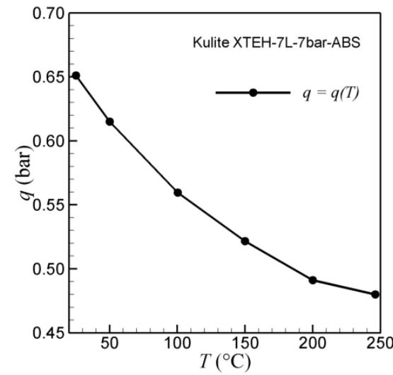
Thermal drift  $\rightarrow (P, T)$  calibration
